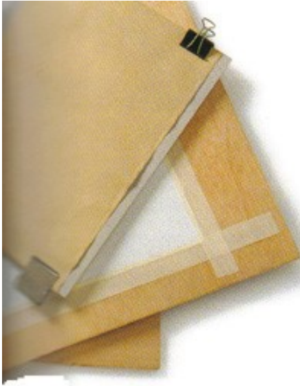
Thumbtacks, clips, and masking tape can all be used to attach the paper to the board.
