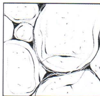
Caps in stacked stone, with or without mortar
